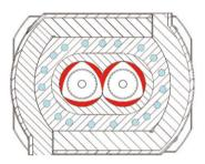
Uniformly distributed cooling channels and heating elements are accurately adjusted to the target processing temperature in each barrel segment.
